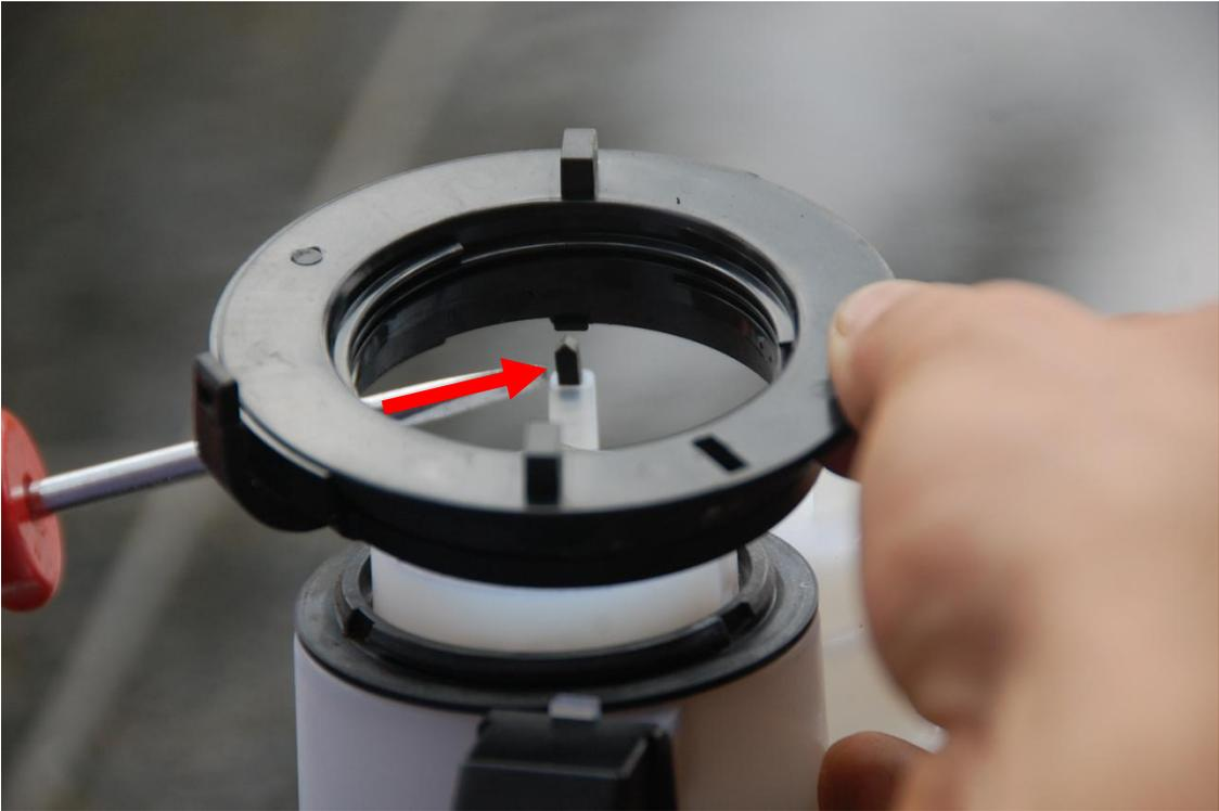
Next, try to rotate the black adjustment ring base (see below). It should not spin freely, but be firm in place.
