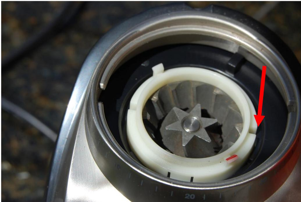
If all looks well, rotate the black adjustment ring counter clockwise until it stops. It must be in this position to install the hopper. Install the hopper, and try grinding a few beans. If the beans are 'floating' in the hopper OR the unit seems to be working except no grounds are being produced, check out our unclogging tutorial. Call 425 641 1245 if you still are having issues.
