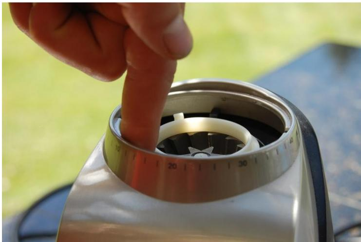
If all that checks out, there is one more thing to verify. With the hopper removed, insert the upper burr (correctly). Then use one of the tabs on the adjustment ring as leverage to rotate it clockwise. The adjustment ring should cover the flanges as pictured.
