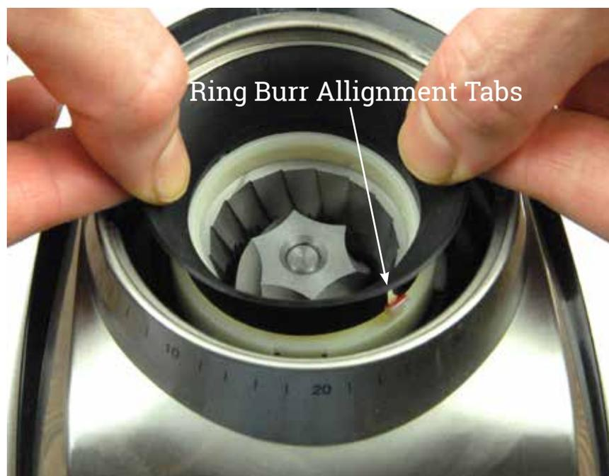
red tab on the burr with the rectangular cutout on the black adjustment ring. Wiggle and push down firmly on the ring burr to ensure that it seats properly. After replacing the burr, replace the silicone seal by lining up the two slots in the silicone seal with the small tabs on the top of the ring burr and slide the seal onto the ring burr.
